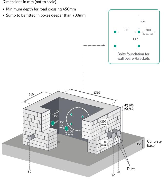
The optional approved pre-formed chamber system Quadbox<sup>™</sup> can be used to speed up the installation process and bring significant productivity benefits as there is no need for specialist box building teams and concrete backfill to be used.
